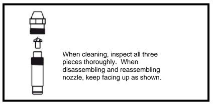
Figure 38 – Nozzle Assembly Detail
